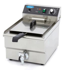
Deluxe single tank fryer Complete with oil valve Very nice finishing Completely made of stainless steel With cold zone Protected heating elements Adjustable thermostat: 0°C to 200°C Overload protection Stands on four rubber feet Tank capacity: 18 liters Min. oil quantity: 13.5 Liters Max. oil quantity: 16 Liters Basket Dimensions: H120 x W235 x D255 mm
